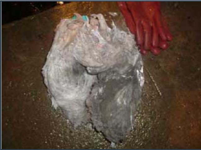
Figure 2 and 2a – Details the compactness of the blockage material; indicative of compounding over time.
